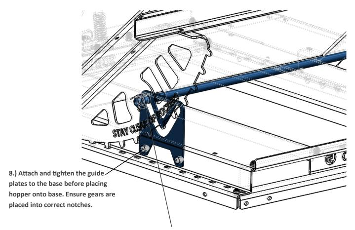
9.) To secure the guide pipe, insert the blue washer then insert the split pin at the end of the guide pipe. (Shown above.) After inserting pin tighten all other bolts previously left loose.
