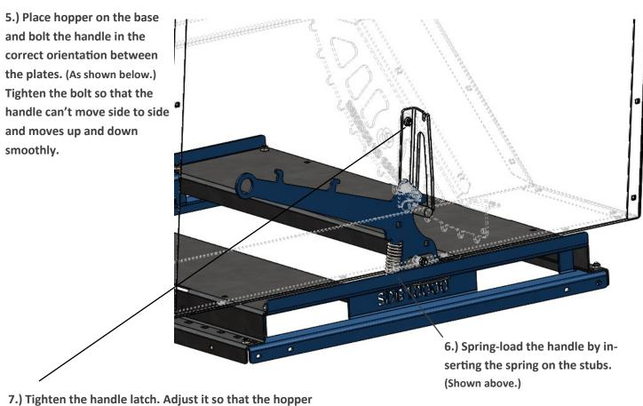
7.) Tighten the handle latch. Adjust it so that the hopper is held securely to the base after locking the hopper.
