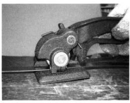
2. Compress the Handle (#1) to lift Support Frame (#8). While in this position, move the tool and slide the strap into the gap below the Feedwheel (#12). The strapping material is now locked and ready to be tightened.
