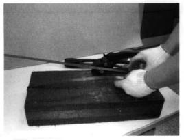
Place the strap around the object you wish to secure as shown. The end of strap is underneath.
