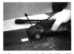
Compress down the Handle (#1) to lift the Feedwheel (#12). Slide the tool away from the strapping material. Cut excess strap with a steel strapping cutter (not included).
