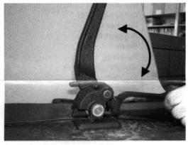
3. Hold the tool with your left hand and pump the Handle (#1) until the straps are sufficiently tight. Don't overtighten the straps as damage may occur to the tool and object being strapped.
