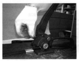
4. Press the Handle Pawl (#4) down so that the Handle (#1) can be released. Place the seal (not included) open side down over both straps in front of the tool.
