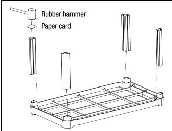
**STEP 1**: Insert Aluminum tubes into the slots on the bottom side of the top shelf using rubber mallet.
