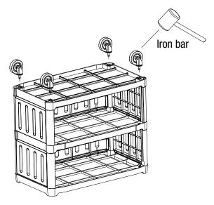
**STEP 4**: Position swivel casters into the caster holes on the bottom of the utility cart and hammer into place.
