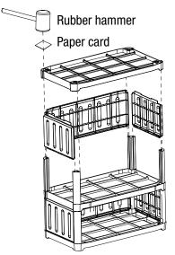
**STEP 3**: Repeat Steps 1 and 2 with remaining tubes, shelf and side panels. Then, mount bottom shelf of the cart onto the aluminum tubes and hammer them into position (see above).
