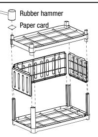
**STEP 2**: Insert (2) short side and (1) long-side panel into the rails on the aluminum tubes. Place middle shelf flat-side down and hammer into aluminum tubes. (See figure above).
