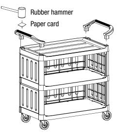
**STEP 5**: Flip the utility cart upright and install handles using rubber mallet by lightly tapping the handle into the handle holes on the top of the cart.
